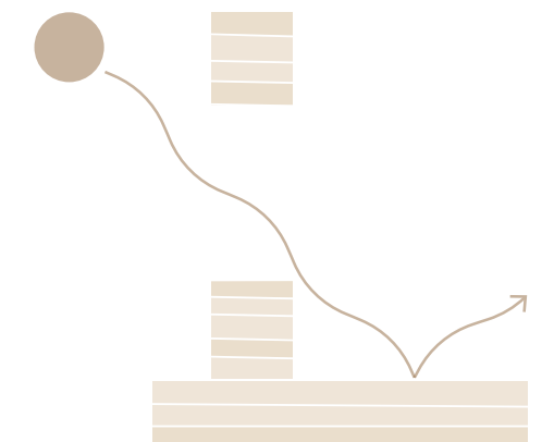
rammed earth has high thermal mass
