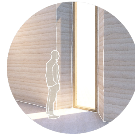
the sculptural qualities of rammed earth enable monolithically slanted window reveals...
