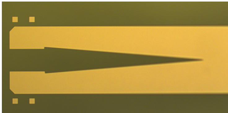
Figure 5.5: Microscope photo of TiN layer, after step 3) in the process.
