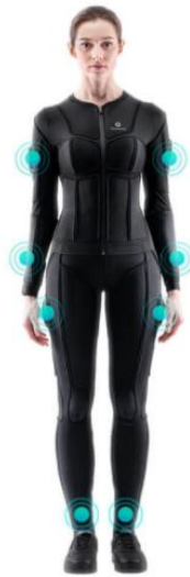
Figure 3.20: Front view of sensor placement for a Teslasuit with 10 IMU sensors [42].
