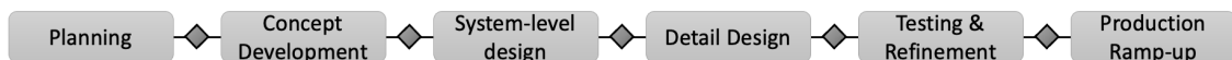
Figure 2.1: Typical process flow diagram for a generic product development process inspired by Ulrich et al. [32].
