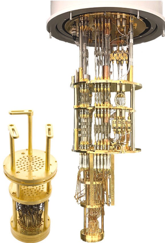
Figure 1.7: SCALINQ’s LINQER on the left and a depiction of its installation in a dilution refrigerator on the right. The image is generously provided by SCALINQ and the use of this image is authorised by SCALINQ [31].
