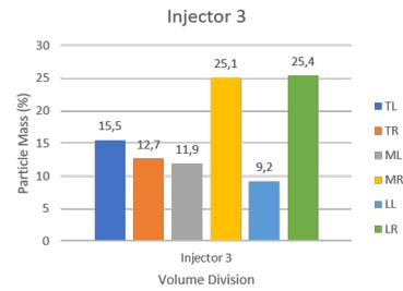
**Figure 4.18:** Particle distribution of injector 3
