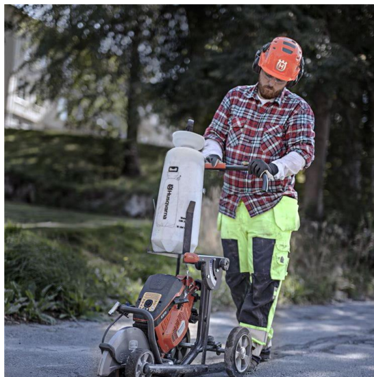
Figure 4: A trolley from Husqvarna to combine with a power cutter
