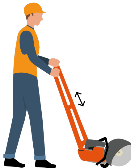
Figure 59: Alternative 6C of the extendable handle
