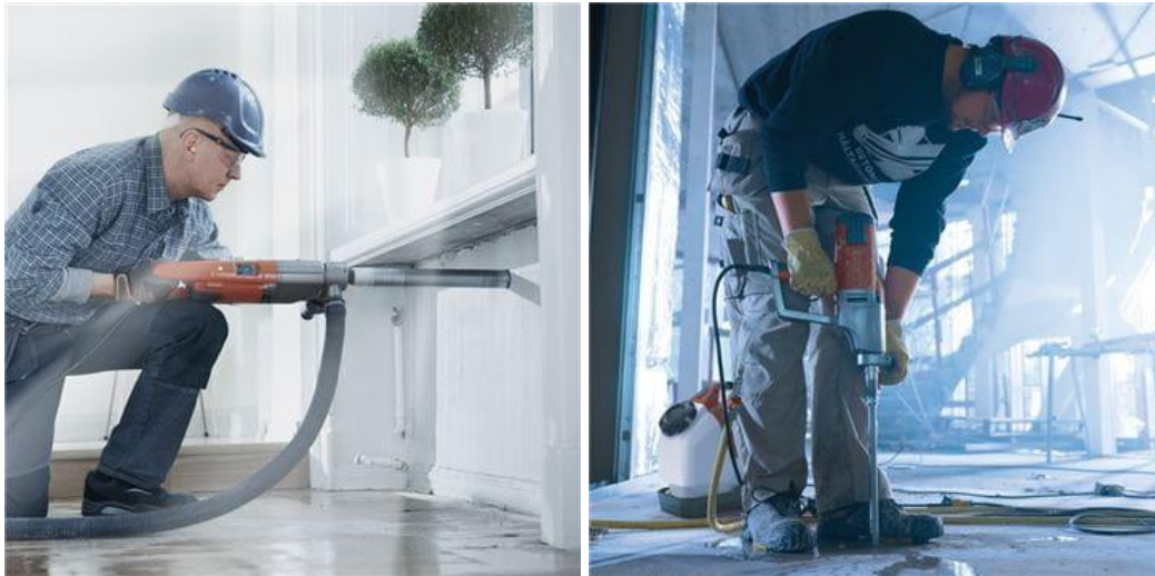
Figure 5-6: Two examples of core drilling machines Husqvarna Construction, (n.d.-d), reprinted with permission
