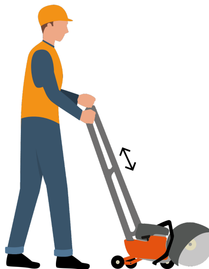
Figure 57: Alternative 6A of the extendable handle
