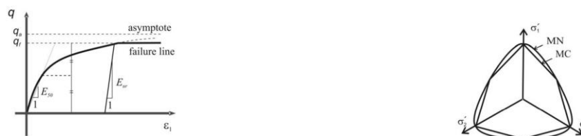
Figure 30 a) Hyperbolic stress-strain relationship, (b) Matsuka-Nakai (MN) and Mohr-Coulomb (MC) Failure criterion (Vogler, 2008).
