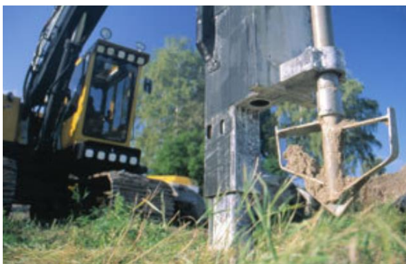
Figure 8 vertical mixing tool (Alén et al., 2005a)
