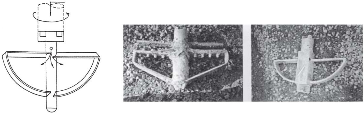
Figure 9 Principle sketch of the traditional mixing tool with semi-circular stirrup and tapered blades and some other examples of mixing tools (Larsson, 2006)
