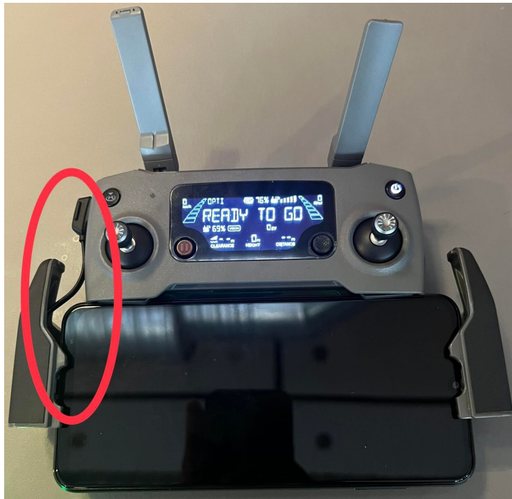
Figure 2.2: Picture of the mobile device connected to the RC via an USB cable (highlighted in red). Source: Primary
