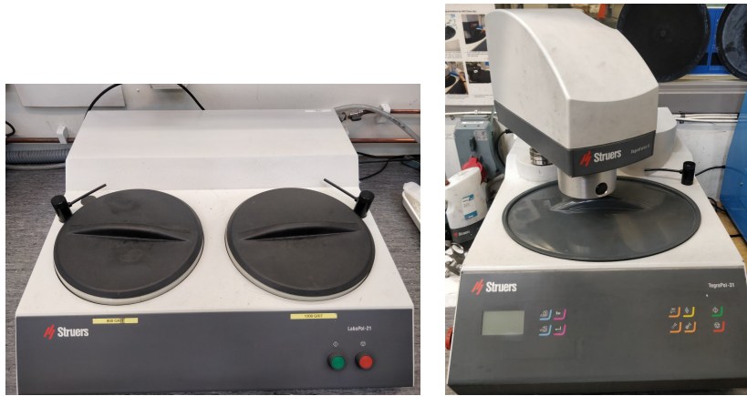
Figure 3.5: Manual grinding machine: Struers Labopol-21 (left) and automatic polisher: Struers Tegrapol-31 (right) used in this study.
