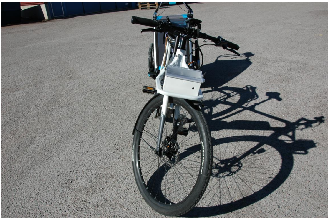
Figure 3.3 Bicycle and trolley with mounted equipment, front view (Leif Sjögren, 2019-04-01).
