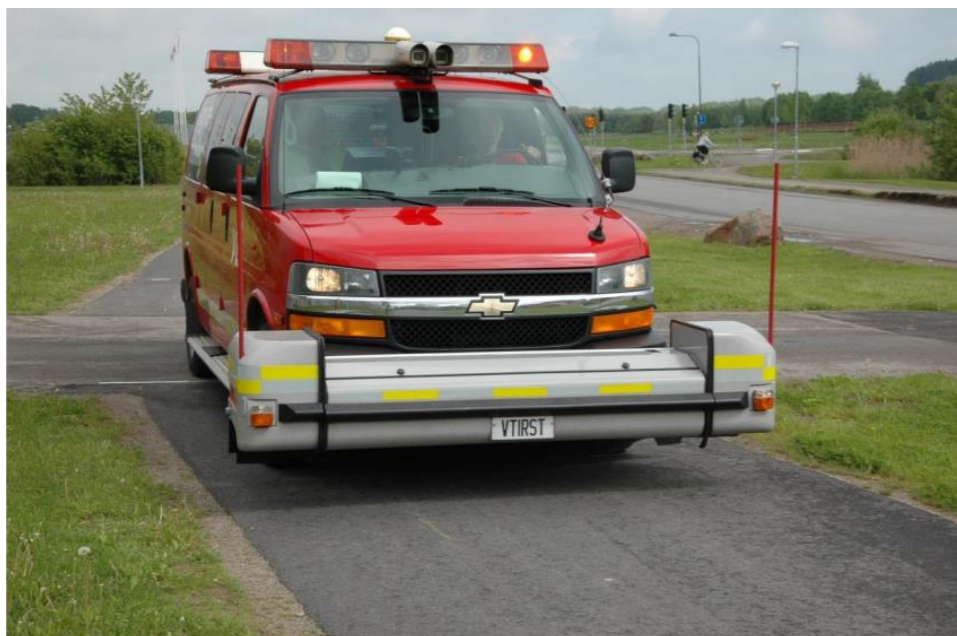
Figure 2.5 Measurement with VTI's laser RST (Niska & Sjögren, 2014).
