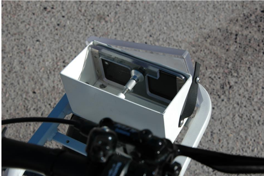
Figure 3.4 Box for mounting of smart phone (Leif Sjögren, 2019-04-01).
