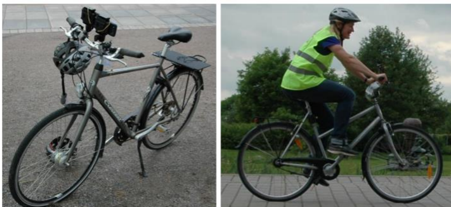
Figure 2.4 Measurements with an accelerometer in a smart phone mounted on a bicycle (Niska & Sjögren, 2014).
