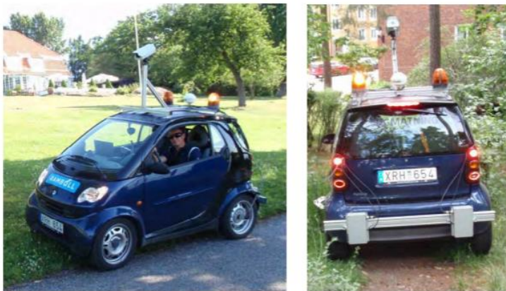
Figure 2.8 Smart car, equipped with two laser sensors (Niska, Sjögren & Gustafsson, 2011).
