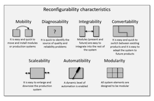
Figure 2.4: Reconfigurability characteristics based on [Rösiö, 2012].
