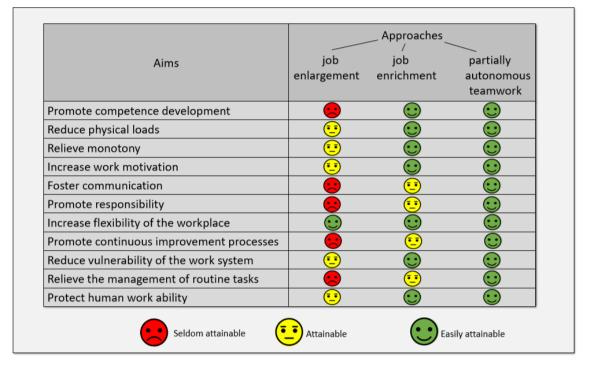
**Figure 6.8:** Approaches and aims of work structuring based on [Wiendahl, H., Reichardt, J., Nyhuis, P., 2015]. The figure illustrates how effective different approaches are for attaining different aims.
