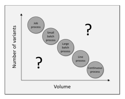
**Figure 5.1:** The Product Process Matrix. The figure illustrates common production process choices, based on the number of variants as well as the volumes to be produced. Figure based on [Hayes and Wheelwright, 1984]
