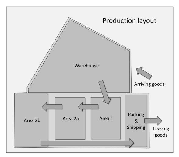
**Figure 6.5:** Layout of the new facilities. The arrows indicate the flow of materials and products through the production system.
