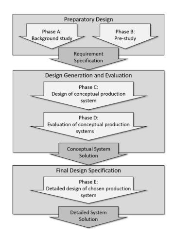
**Figure 3.1:** Adaptation of the systematic method for production development originally suggested by Bellgran [Bellgran, 1998]. Parts of the original method related to investment and development planning, realization and start-up have been omitted as they fall outside of the scope of the thesis.
