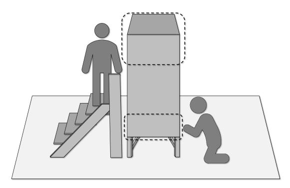
**Figure 4.10:** Extreme working positions. The most extreme work positions are performed at the top and the bottom of the product, indicated in the figure with dashed lines.
