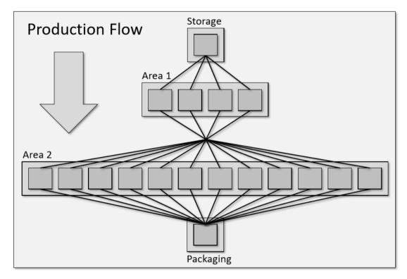
**Figure 4.1:** Conceptual illustration of the current production flow. The large difference in number of work stations between Area 1 and Area 2 is due to a larger work content and longer lead times in Area 2.
