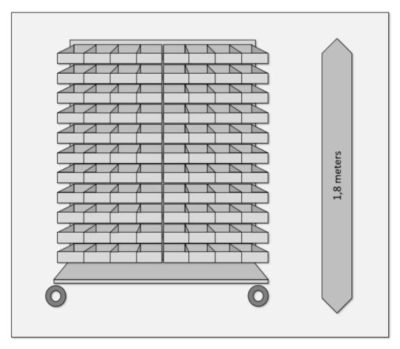
**Figure 6.2:** Bin racks for line stocked components. The racks fit many small bins for components such as screws and washers.
