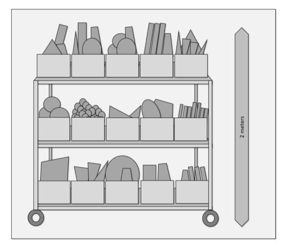
**Figure 4.6:** Kit cart for assembly in Area 1. Different boxes contain components for individual assembly operations. The contents of the boxes are unstructured.
