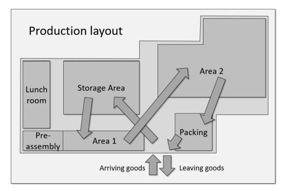
**Figure 4.2:** Layout of the current production facility. Arrows indicate the flow through the production system, from the arrival of central components such as chambers and framework to the final packaging and departure of finished products.
