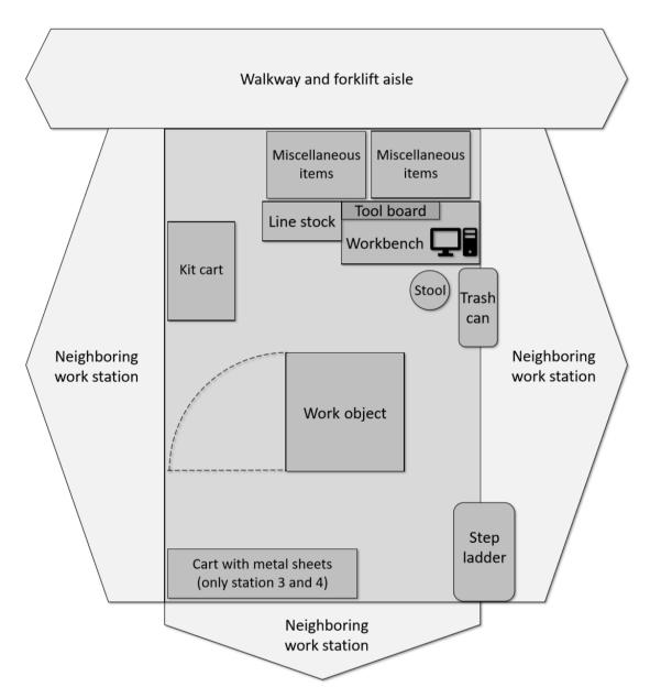
**Figure 6.3:** Proposed workplace design. Each work station includes some extra space for miscellaneous items. This can be used either for specific components necessary at a certain work station, or for general objects needed in Area 1.
