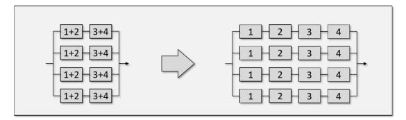
**Figure 6.1:** Division of work blocks between stations. In the initial design, each work station will include 2 work blocks. In the final design each station only contain 1 work block.
