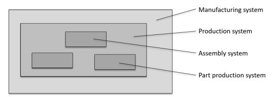
**Figure 2.2:** Hierarchical perspective of production systems based on [Bellgran and Säfsten, 2010].
