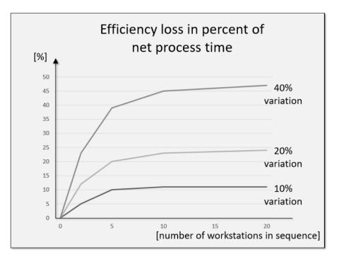
**Figure 5.3:** Efficiency loss due to intra-station variation based on [Engström et al., 1996]. The figure illustrates how efficiency losses depend on the intra-station variation as well as on the number of work stations.
