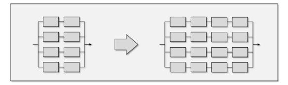
**Figure 5.4:** Proposed flow principles. 4 parallel lines that each contain 2 serial work stations is suggested for the initial design. This is then suggested to be increased towards a flow of 4 parallel lines with 4 serial work stations each.
