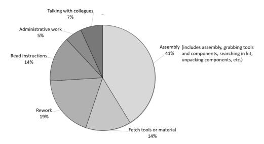
**Figure 4.4:** Time distribution between different activities in Area 1. Work sampling was performed throughout the assembly of one product. The time distribution shown might therefore not be representative of what is typical. It does however give some indications of how time is spent.
