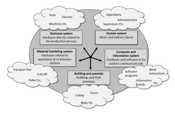
Figure 2.3: Constituent parts of production systems based on [Rösiö, 2012].
