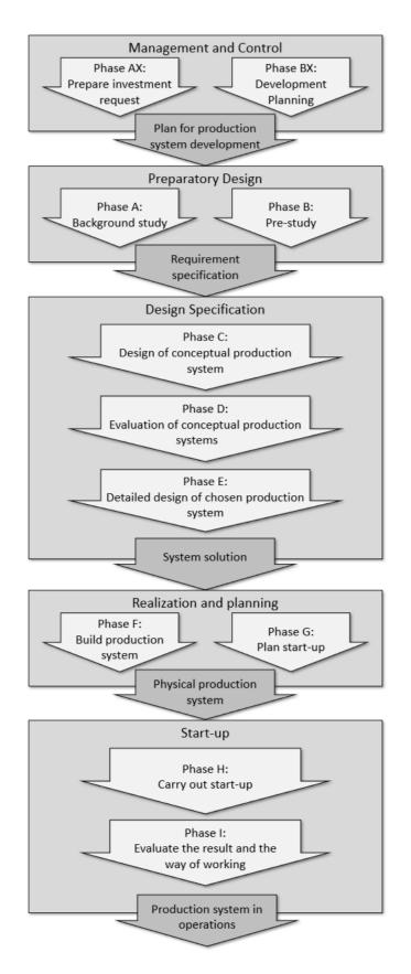
**Figure 2.1:** Systematic method for production system development based on [Bellgran, 1998].
