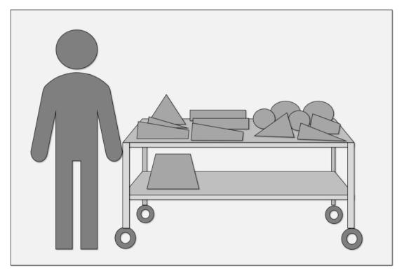
**Figure 6.4:** Future kit example. The figure illustrates a simple kit based on the division of work into 4 work blocks. All or most components are accessible at a ergonomically suitable height.
