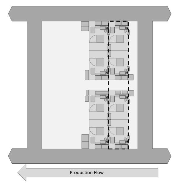
**Figure 6.6:** Detailed proposal for the initial layout. The dashed box illustrates the area covered by the overhead crane.
