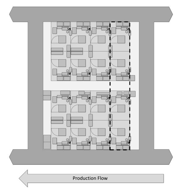
**Figure 6.7:** Detailed proposal for the final layout. The dashed box illustrates the area covered by the overhead crane.
