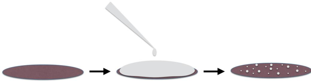
Figure 7. A schematic showing the particle dispersion process. After the PMMA layer on the surface of the substrate is activated and charged by RIE with oxygen and PDDA, respectively, a pipette is used to apply a colloidal solution of PS beads. After rinsing and drying the PS beads remain on the surface.
