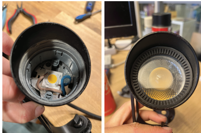
Figure 8.9: The LED chip and the lens
