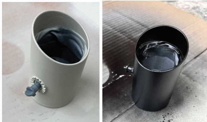
Figure 8.7: First and third layer layer of spray
