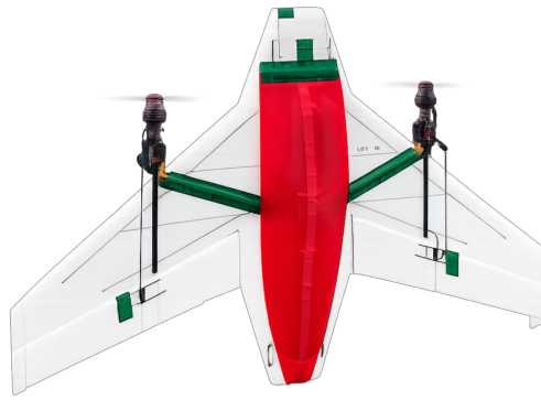
Figure 1.1: Fixed-wing tailsitter UAV developed by Remote Aero
