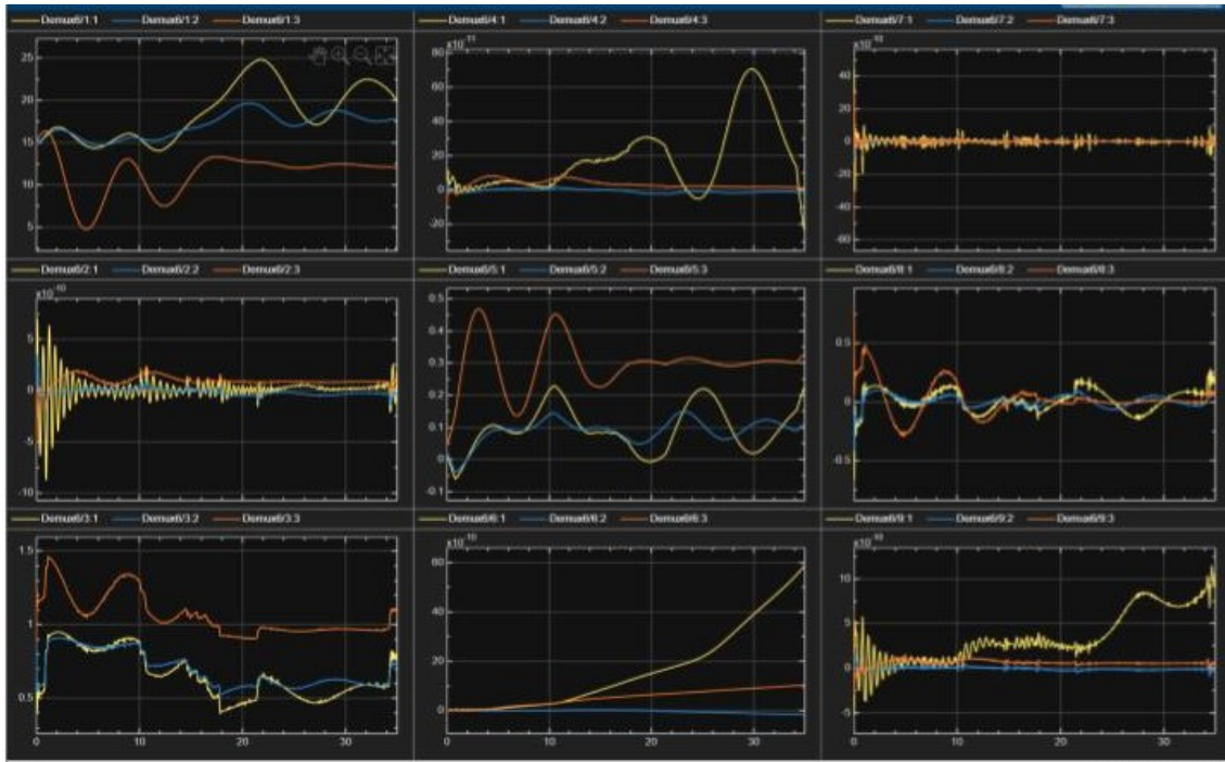
Figure 3.20: NL (yellow), LPV (blue) LTI (orange) - Initial validation of the LPV performed by flying with a joystick.
