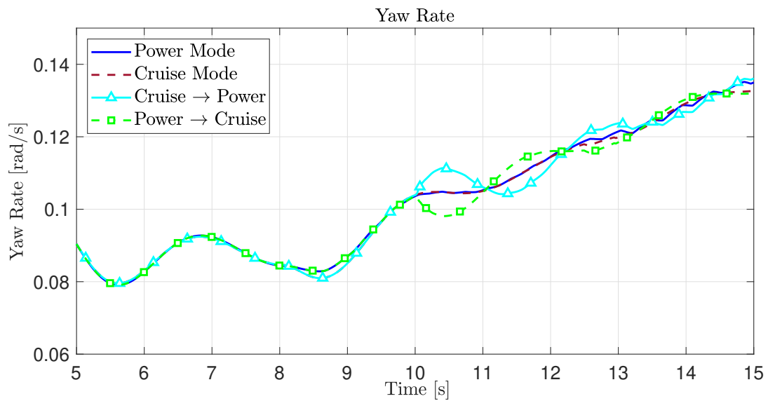
Figure 3.7: Yaw rate over time for mode switching (at t = 10 s) during acceleration while cornering with a simulated driver.
