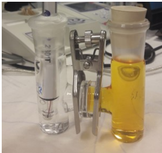
Figure 3.3: Experimental setup for permeation tests.
