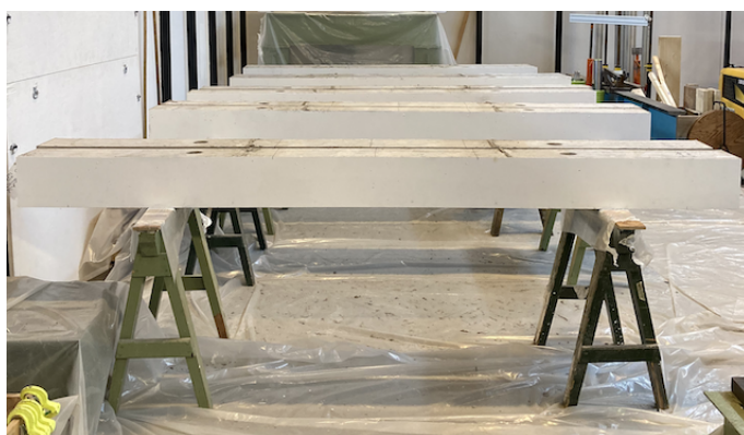
Figure A.10 The beams were painted with a white backdrop to prepare for the DIC.
