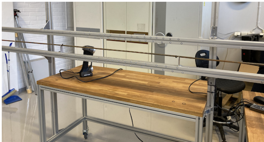
Figure A.2 The setup for the 3D scanning, which shows the frame, 3D scanner and placement of the reinforcement.
