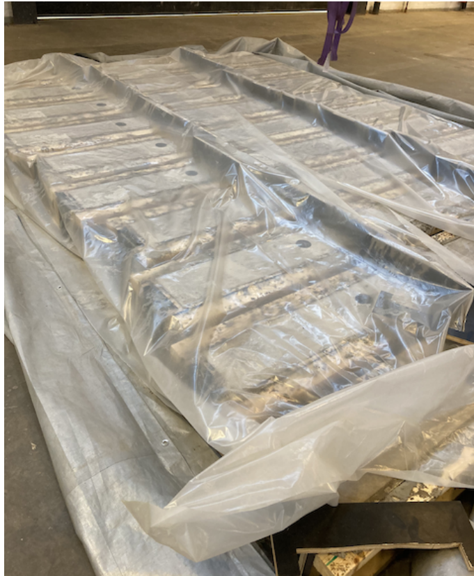
Figure A.9 The beams were stored under plastic sheet to cure.
