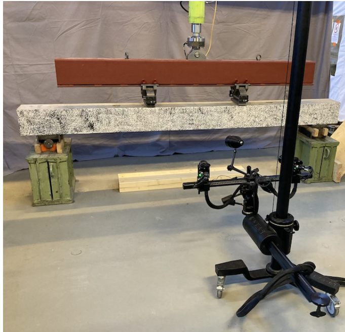
Figure A.13 The static four-point bending test setup with the DIC camera.
