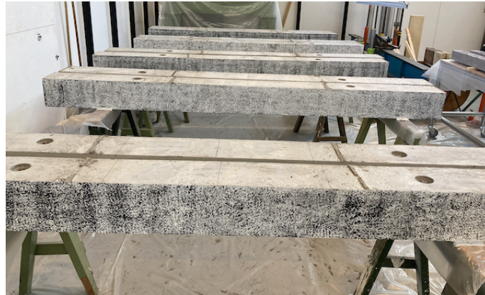
Figure A.11 The white beams were painted with a black speckle pattern to prepare for the DIC.
