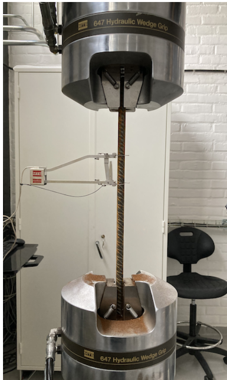
Figure B.6 Steel reinforcement test setup with the extensometer.
