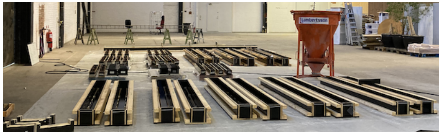
Figure A.5 Preparations of the forms before casting. The ten closest forms were prepared for this thesis.
