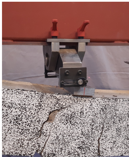
Figure 5.7 Eccentricity of loading point for beam 8 with small loading plate.
