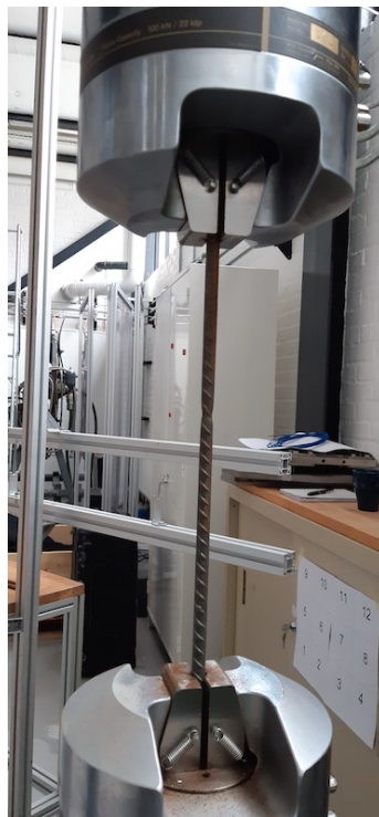
Figure B.7 Example of steel reinforcement necking under tensile strength test.
