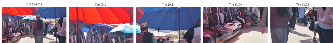
Figure 6.3: Illustration of the tile decomposition strategy used in the self-distillation prototype. A full video frame (left) is uniformly partitioned into spatial tiles (right), each providing a localized view captured by the same camera at the same time step.
