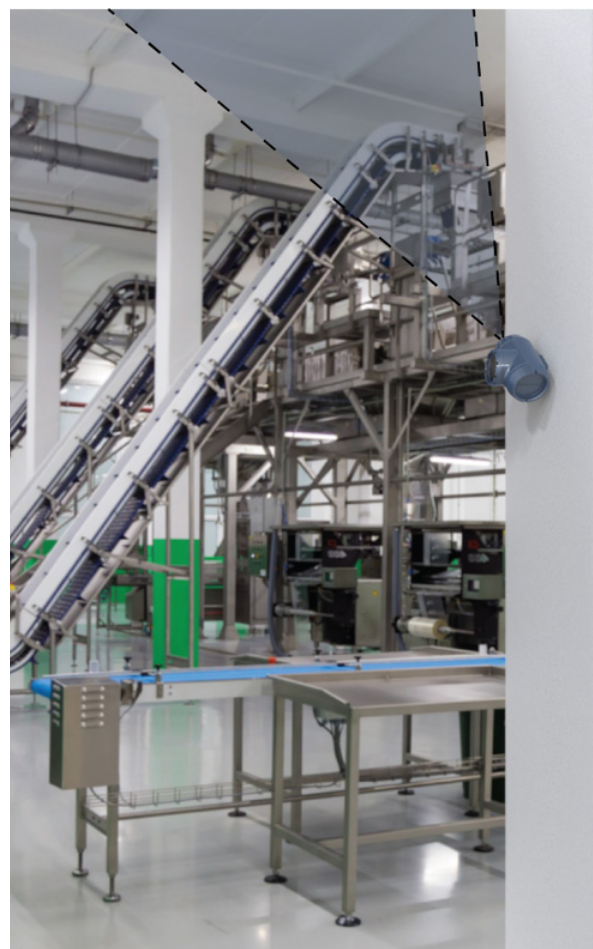
Figure 6.19. The product rendered in a production site measuring vibrations several meters from the ground.
