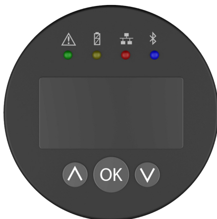
Figure 6.16. The LED lights indicating status. From left: (1) status, (2) battery, (3) wire connection, and (4) bluetooth.
