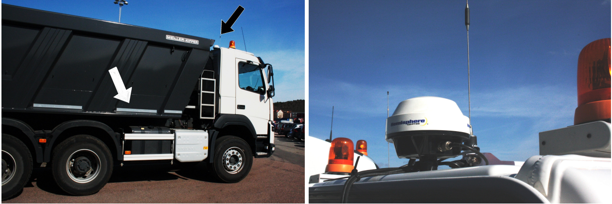
Figure 5.1: The GPS was mounted on the driver's cabin as shown by the black arrow in the left panel. The white arrow points at the location of the IMU. The right panel shows the GPS used at the loggings.
