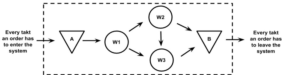
**Figure 16: Generalized takt time control (Slomp et al., 2009)**
