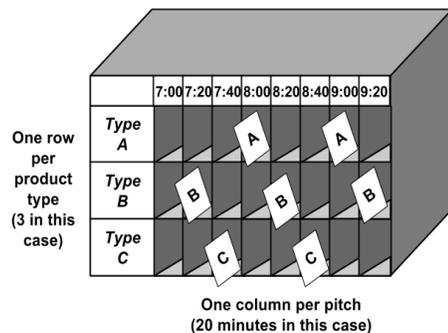
Figure 18: Load Leveling box (Rother & Shook, 2003)
