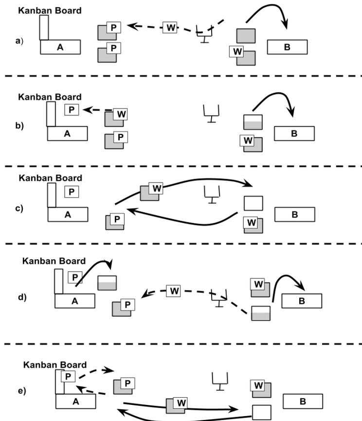
Figure 13: Two card kanban (Adapted from Wånström, 2015)
