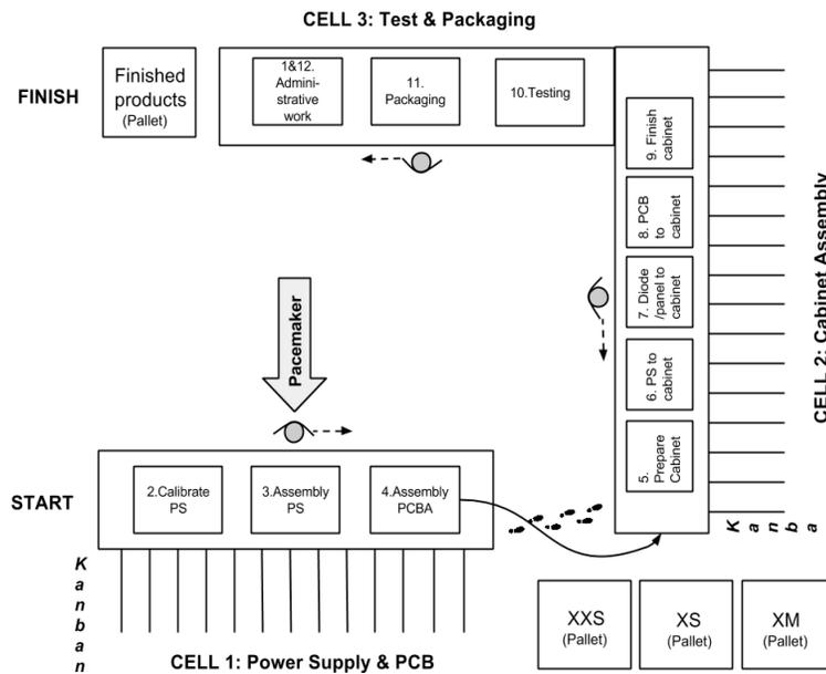
**Figure 29: Scenario one, all operators inside the U-layout**
