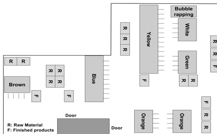
**Figure 25: Milletechnik's production layout**
