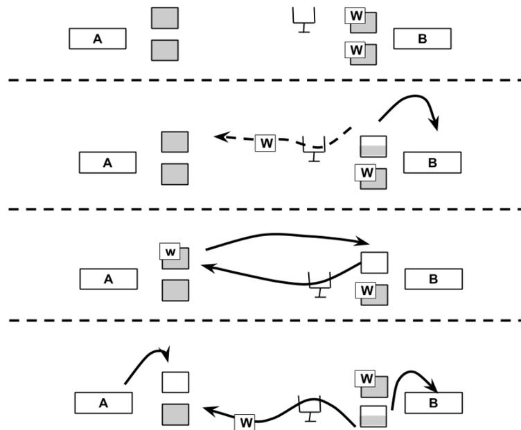
Figure 14: One card kanban (Adapted from Wånström, 2015)
