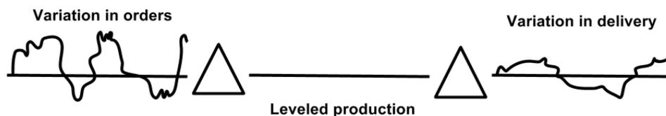
Figure 17: Leveled production (Adapted from Wänström, 2015)
