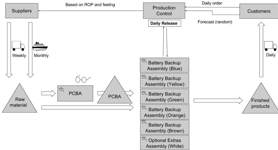
**Figure 22: Value stream mapping (VSM)**
