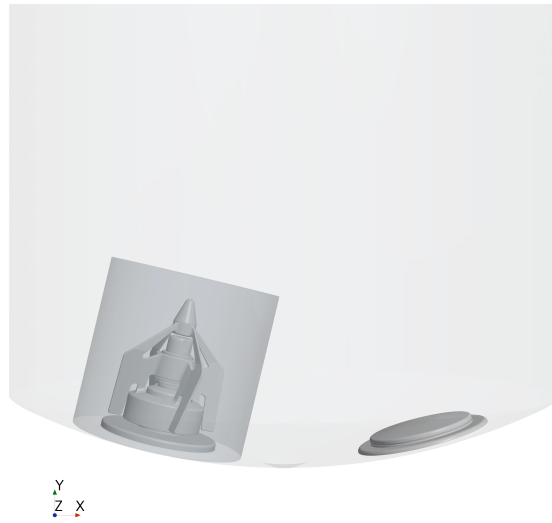
Figure 3.2: Positioning of the rotating zone within the tank geometry. This region encloses the impeller and is used in both MRF and SM simulations to model impeller motion.
