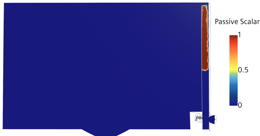
Figure 3.16: Initial tracer fluid location on a plane intersecting the center of the draft tube.
