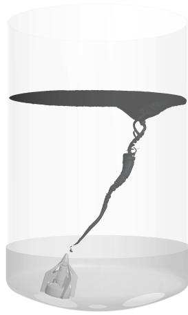
Figure A.2: Time-averaged vortex surface from the transient FVM simulation at 268 RPM.
