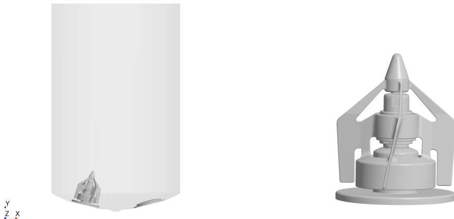
(a) Geometry of the tank in case 1 in the XY-plane. The tank is cylindrical and the impeller is positioned near the bottom and offset from the center.
