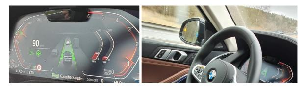
Figure 4.4: BMW X6's traffic situation display. Figure 4.5: Blind spot indicator
