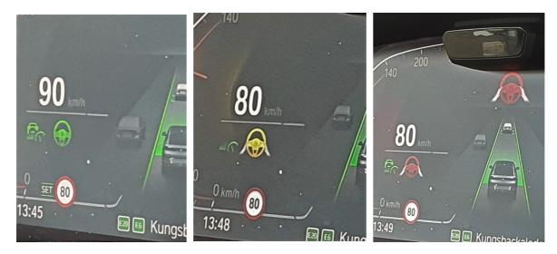
Figure 4.8: Green symbol when AS is activated. Figure 4.9: Yellow symbol with hands on wheel. Figure 4.10: Red symbol with hands on wheel, both to the left and in the middle of the display.
