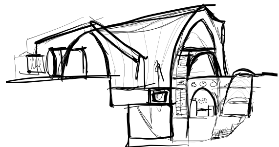
Early sketch of a habitat similar to the final design where the 3D printing arm would lift objects into an airlock for experiments, allowing the crew to move heavier experiments and equipment into the habitat.
