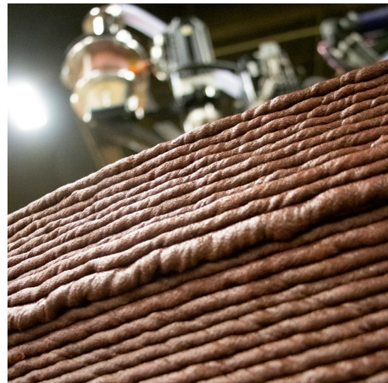
Figure 2. Printing Closeup (AI Space Factory 2019) Reprinted with permission. Test prints of a simulated regolith/PLA mixture by AI Space Factory.
