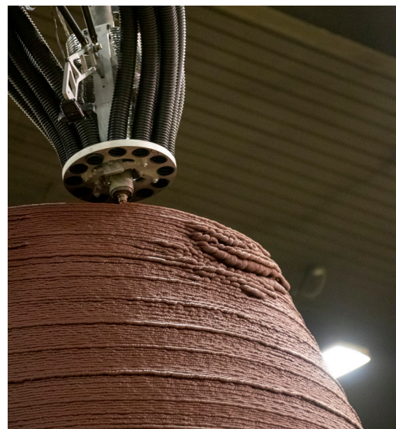
Figure 3. 3D Printing (AI Space Factory 2019) Reprinted with permission. Test prints of a simulated regolith/PLA mixture by AI Space Factory.
