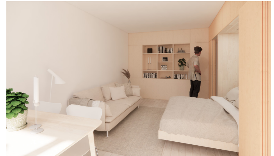
Figure 128. Illustration of main room, with a foldable bed, integrated in the Living Box. When the bed is folded and hidden, it gives more free space in the apartment during daytime.
