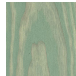
Figure 11. Linseed oil treatment on plywood
