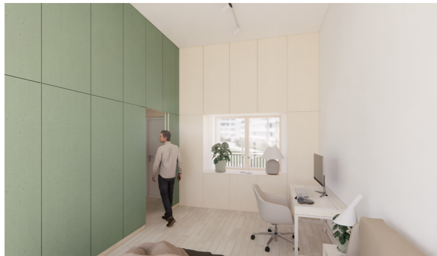
Figure 109. Illustration of the two-room apartment with Living Box I, and access balcony, that allows daylight from two directions. The window is integrated in the built-in storage in the exterior wall.
