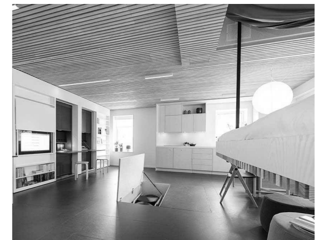
Figure 18. Interior of the Dream Home in Linköping. Storage under the floor, bed hanging from the roof, and movable walls.
