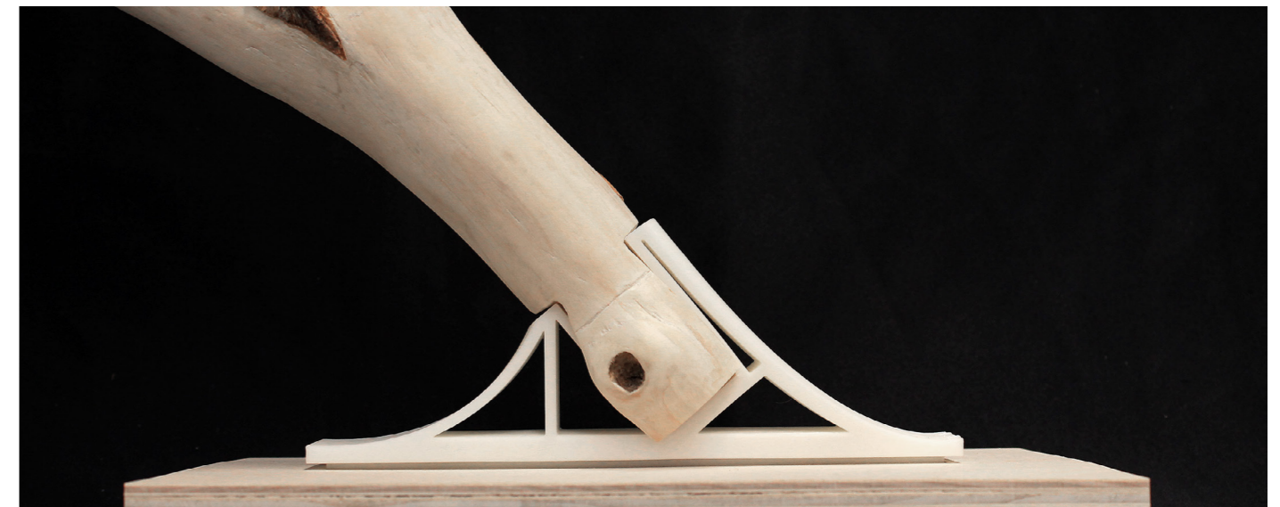
Fig. 67. Milled piece of tree fork attached to base.
