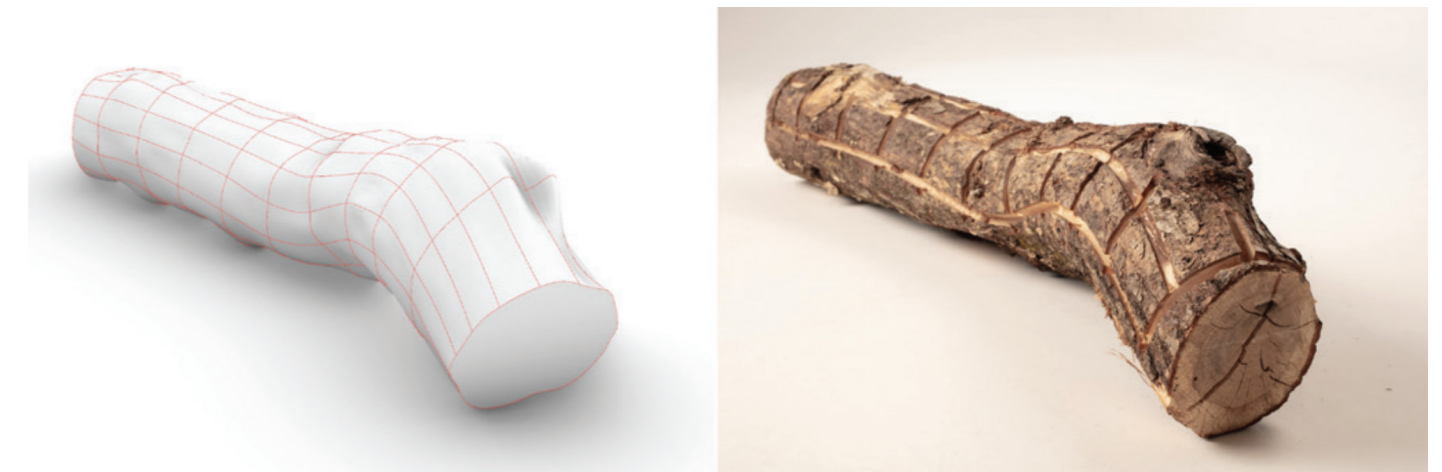
Fig. 14. A 3D model of a log with isocurves (Left). Physical log with milled isocurves (Right).
