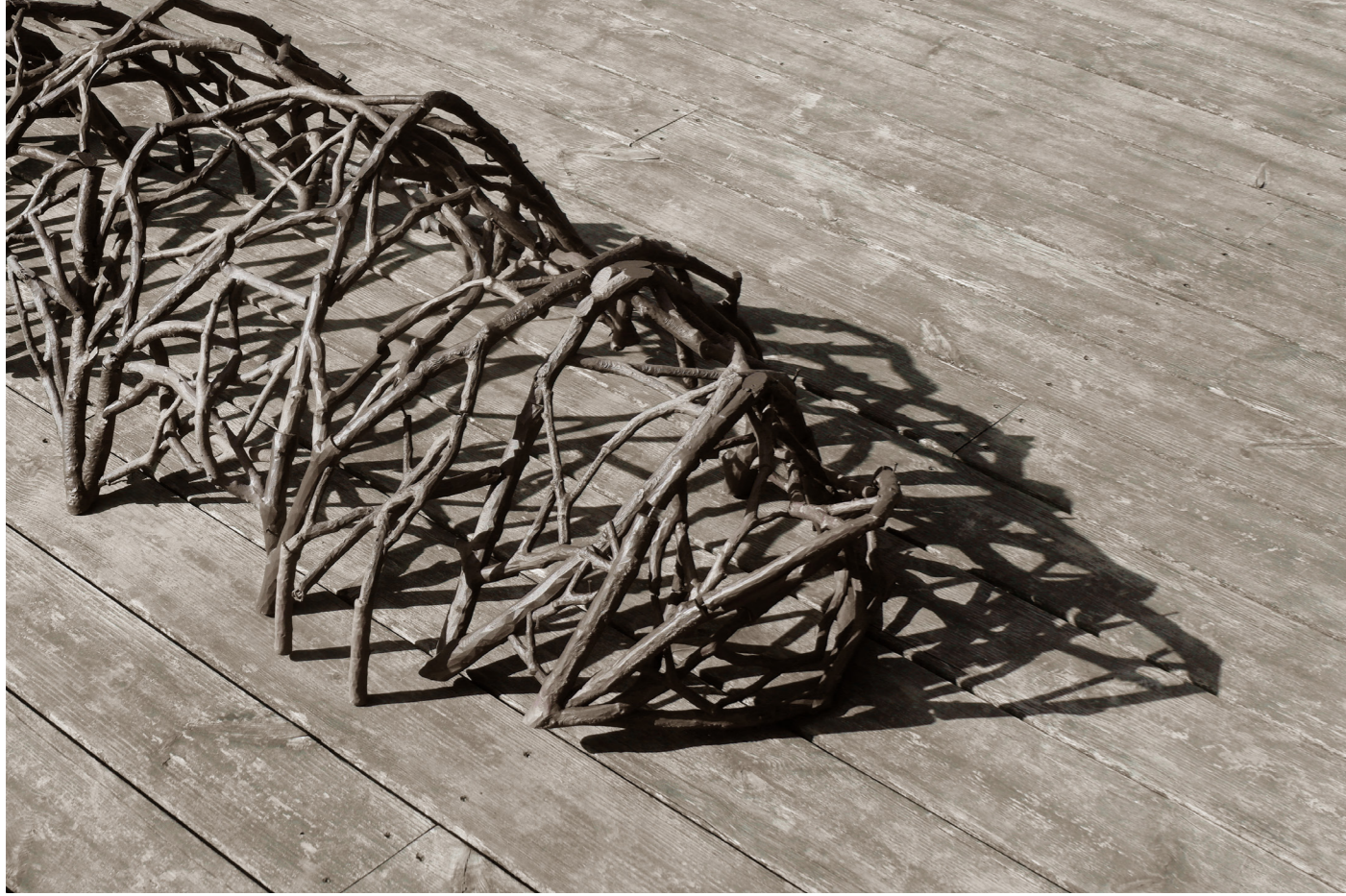
Fig. 51. Prototype 4. Structure Model. Physical raw wood pieces were 3D, and the resulting models were 3D printed in 1:25 scale.
