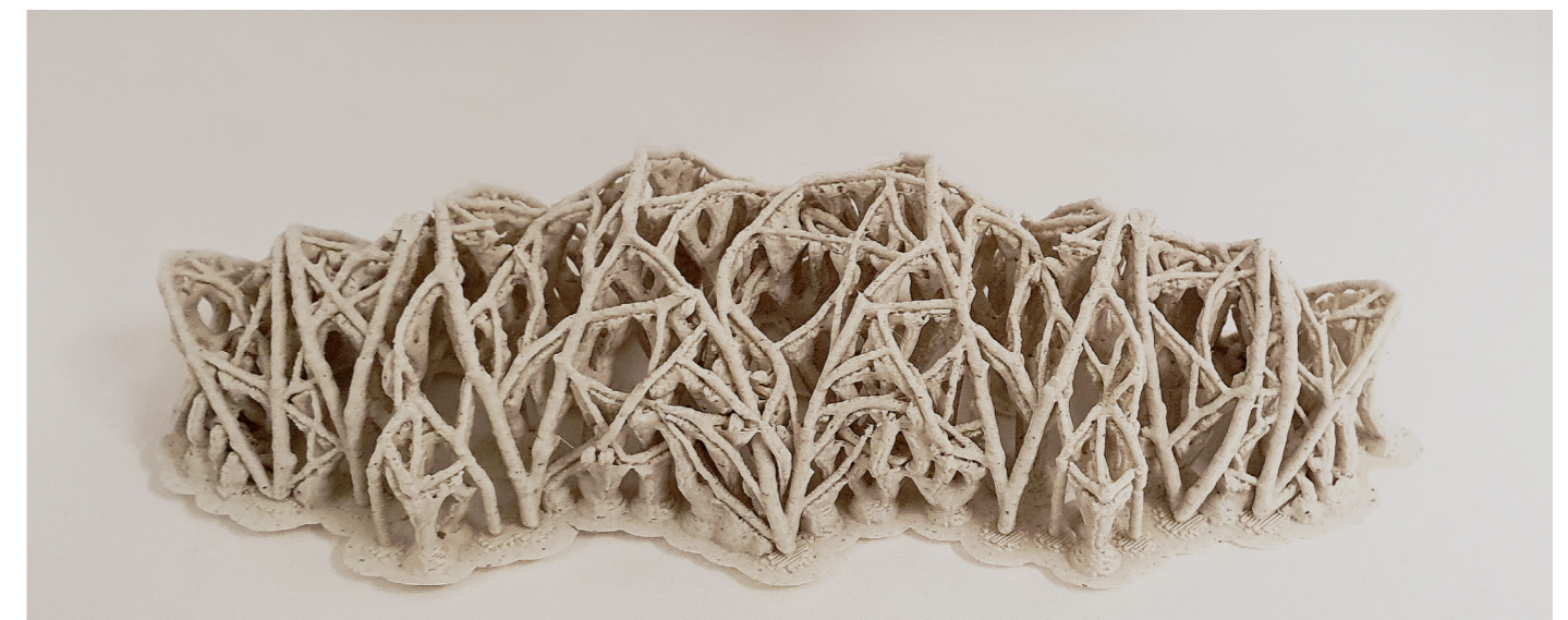
Fig. 50. Prototype 4. 3D printed model with organic support unremoved in 1:200 scale.
