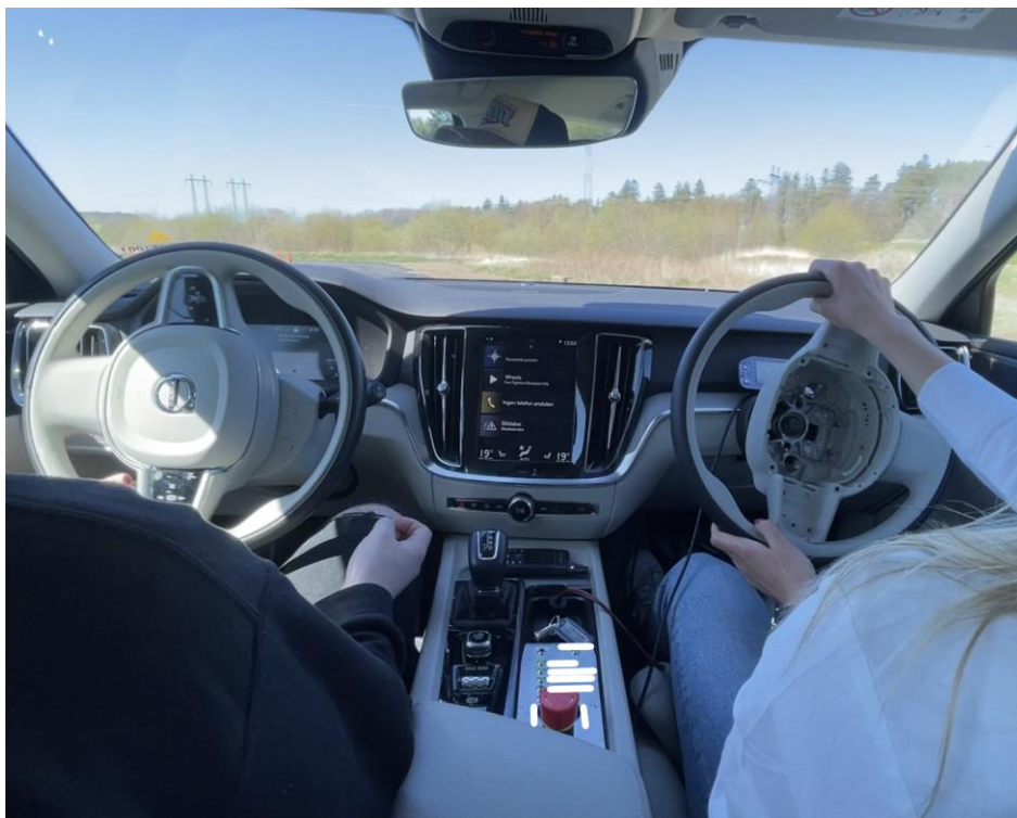
Figure 3.3. The test vehicle used where two steering wheels are installed. One with SbW and one with a steering column. A controller unit is also included between the seats.
