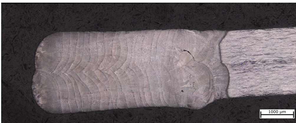
Fig. 16. Enlarged image of the first cross section in Fig. 15 showing voids/cracks in the initial layers where SS308LSi and Inconel 718 are mixed.
