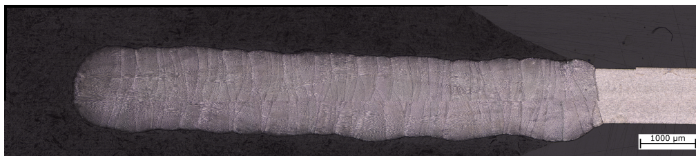
Fig. 12. Cross sectional image of a etched single bead on supported wall sample.
