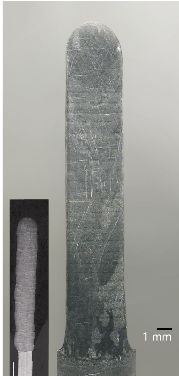
Fig. 20. Comparison of cross section scans from single bead walls created by the new tool in SS308LSi and old tool in Ti6Al4V. Comparison sample provided by Procada [3].
