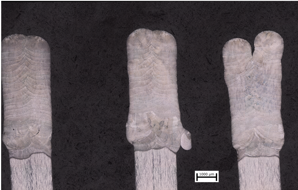
Fig. 15. Three cross section scans of dual bead on supported wall shown in Fig. 14 stitched together.
