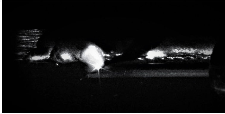
Fig. 7. Process image of a runaway wire. The wire is fed from the right into the melt pool in the center of the image. The wire has deflected downwards in the image resulting in an interrupted process flow. Feed direction is from left to right.
