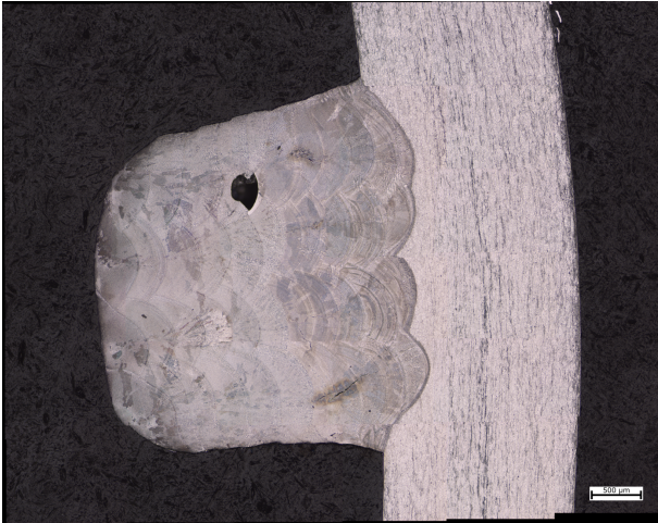
(a) Cross section image of the test coupon showing a void defect around layer 7.
