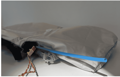
(a) External placement of the SAB pressure probe, coloured in blue.
