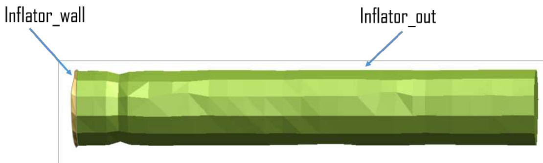
Figure 3.4: Comparison of the original module leakage part, inflator_out , and the adjusted module leakage part, inflator_wall , used in the CPG linear impactor model.
