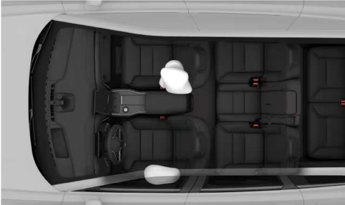
Figure 2.1: Top-down view of a Volvo EX90 illustrating the mounting and deployment of a SAB, designed to protect the occupant’s thorax and pelvis [29].
