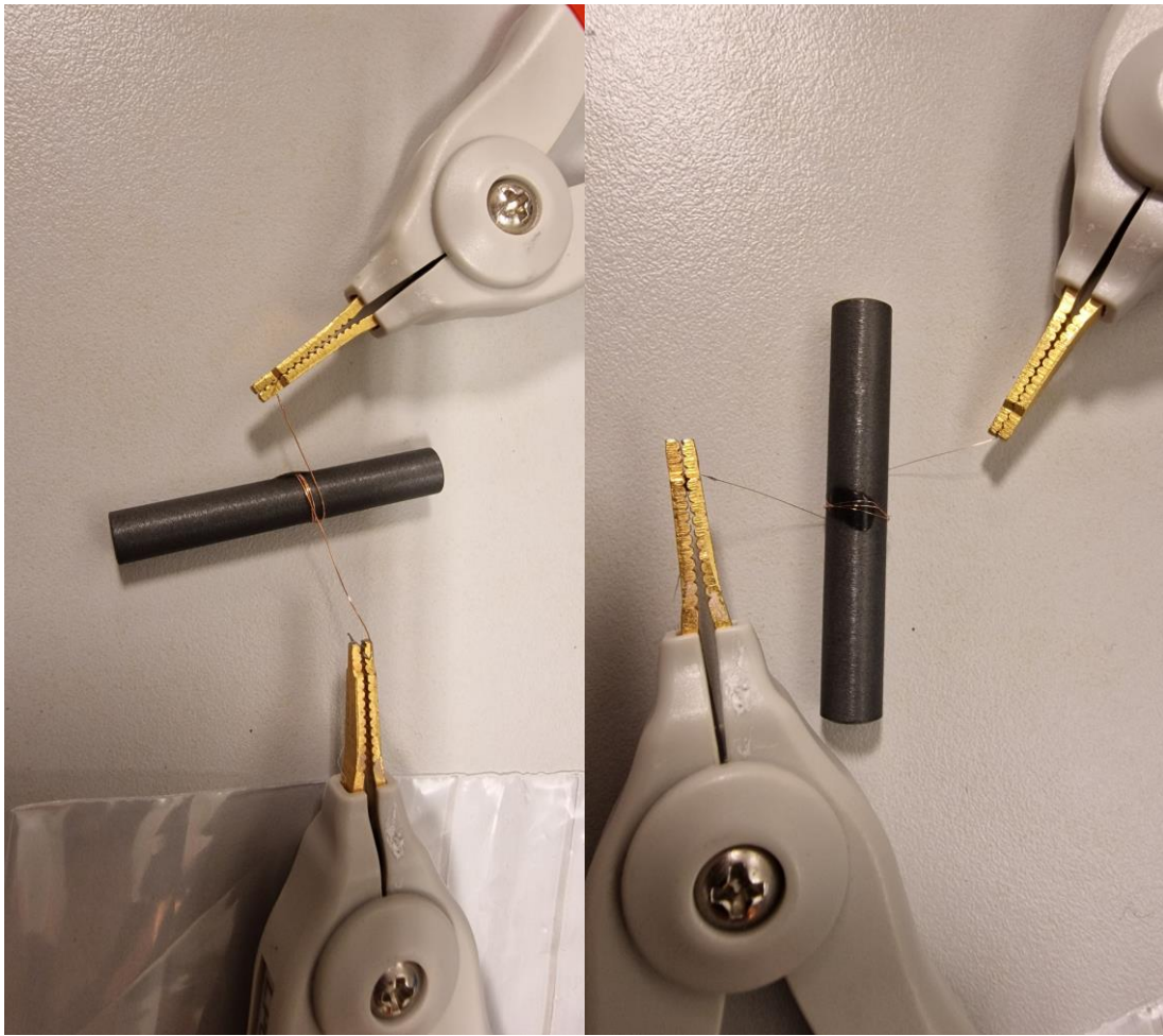
Figure 5.2: Images of the hand-wound ferrite core coils. (A) Prototype A, Relative permeability = 2300, 6 mm diameter, 0.15 mm wire. (B) Prototype B, Relative permeability = 2300, 6 mm diameter, 0.07 mm wire.
