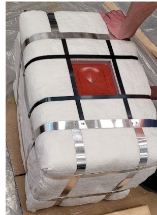
Figure 7: The isolation and metal straps.
