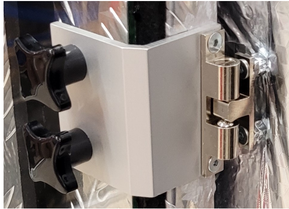
Figure 12: Handle and the lock mechanism.
