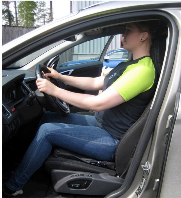
Figure 15: The driver is clashing with the roof when sitting on the foam pad
