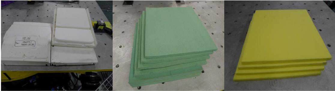
Figure 19: Reference (left) Regufoam Vibration 150 Plus (middle) Sylomer SR11 EN (right)
