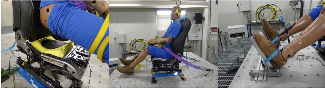
Figure 23: a) Accelerometer placed on test material b) Manikin strapped to the backrest c) Manikin feet strapped to the footrest
