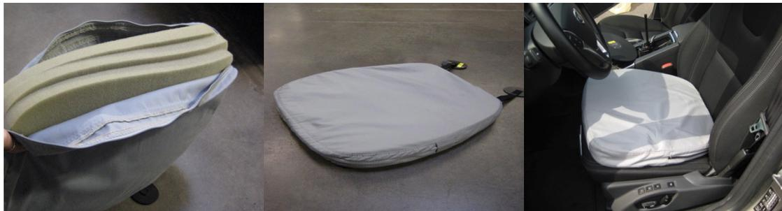
Figure 16: a) Three layers of PUR b) Complete design ready to be installed on the seat c) The pad is installed on the seat
