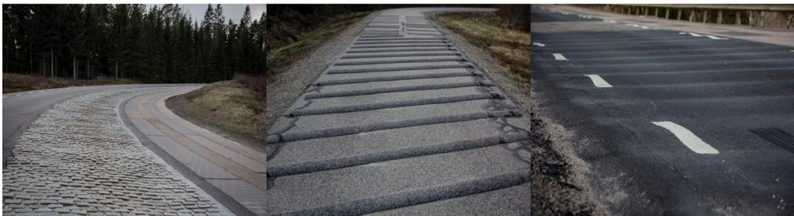
Figure 9: a) Belgian pave (left) b) Silver creek (middle) c) Corrugation (right)
