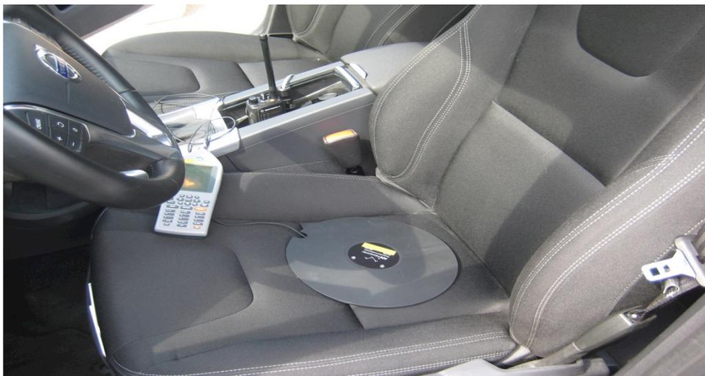
**Figure 6:** The image shows the measuring equipment. The grey device below the steering wheel is the vibration analyzer and the black disc on the seat cushion is the accelerometer
