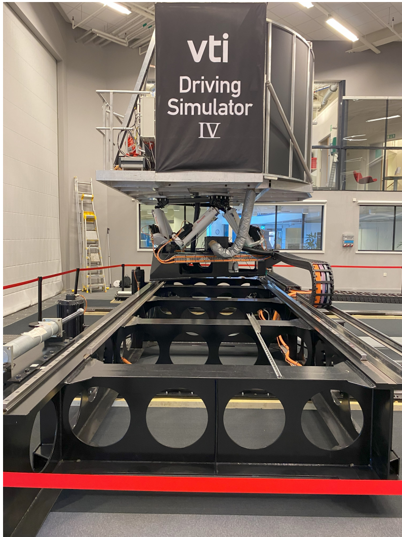
(a) The Y rails of Sim IV
