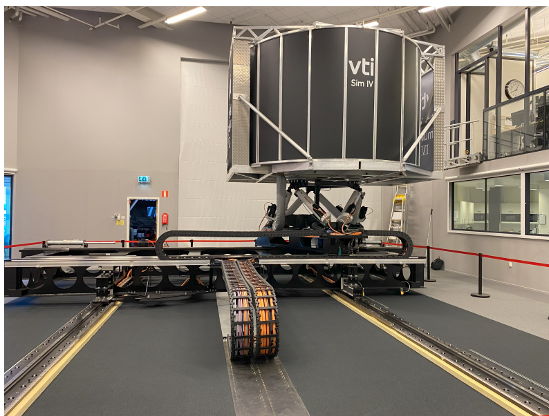
(b) The X rails of Sim IV
