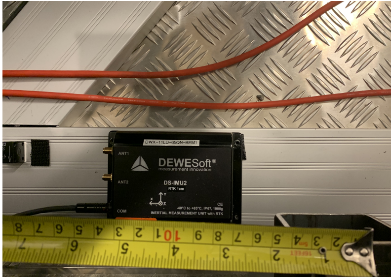
Figure 3.1: IMU placement used by Kumar [22].
