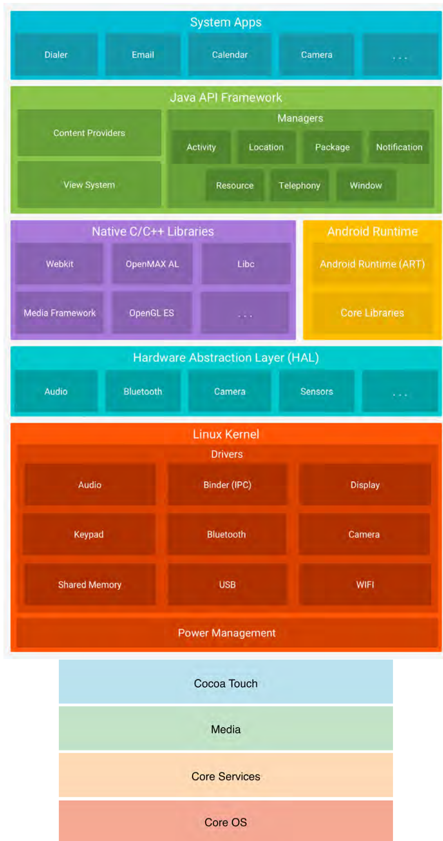
Figure 3.1: An overview of the layered architecture of both Android (on top) and iOS (below). Red indicates close-proximity to hardware.
