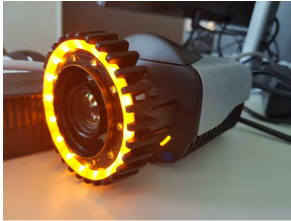
Figure 8.3: A Miqu camera with its LED-ring lit.
