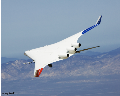
Fig. 2. The X-48B Blended Wing Body research aircraft. From [5].
