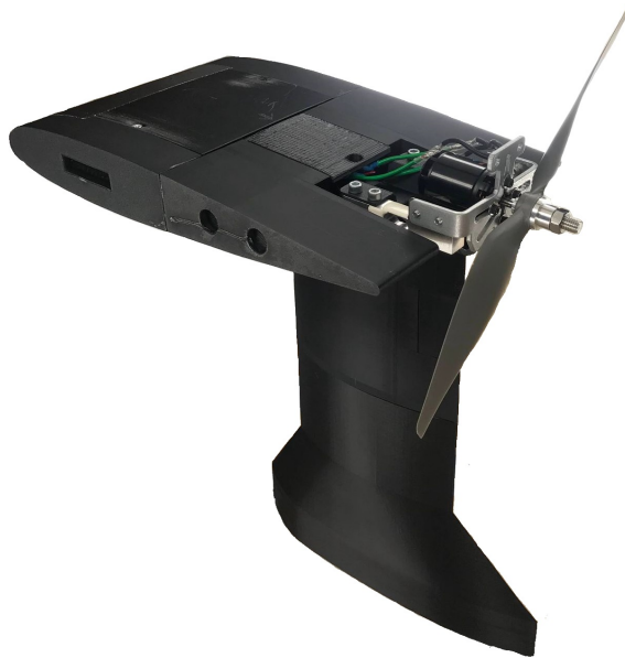
Fig. 9. Fully assembled testing rig with a motor and propeller in place.
