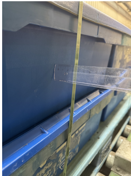
Figure 1.3: Gap between straps and containers.
