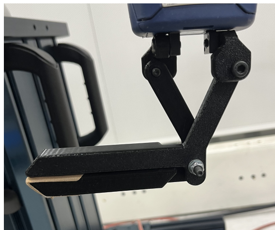
Figure 4.3: 3D-printed end-effector tool (see Sec. 4.1.4), mounted on the SCHUNK Co-act gripper (see Sec. 4.1.2).
