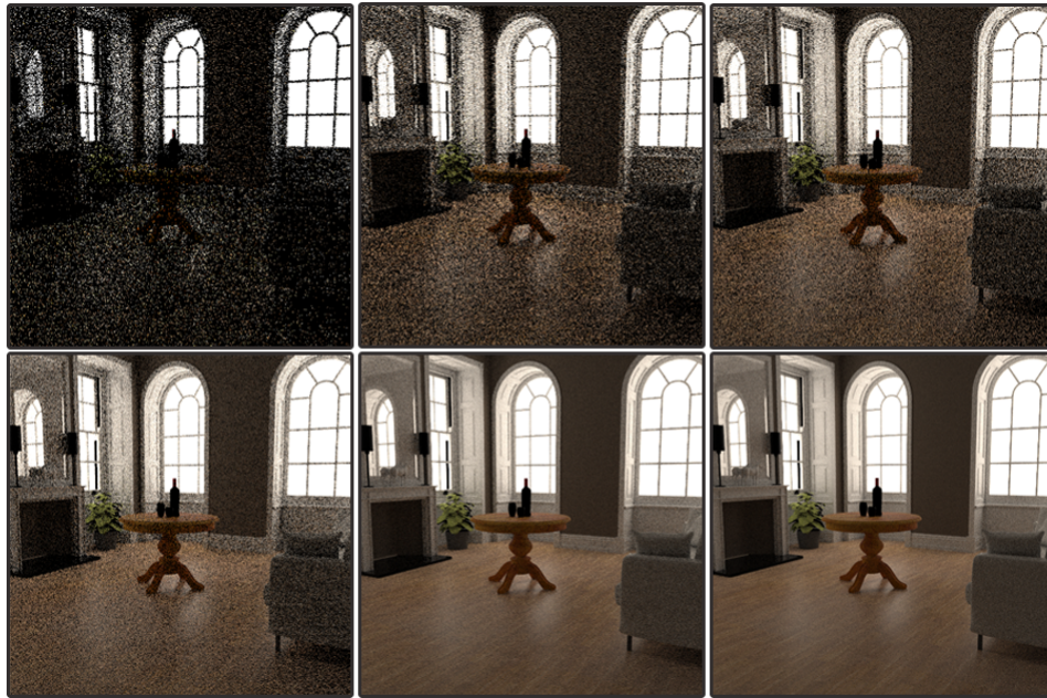
Figure 3.2: Showing different stages of the path tracing process, having traced different amount of samples per pixel. From top to bottom, left to right: 1spp, 8spp, 16spp, 256spp and 512spp
