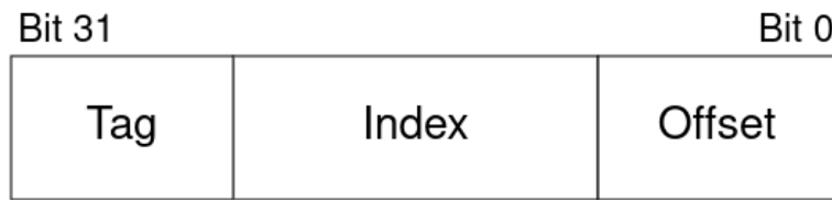
Figure 2.2: The structure of a 32-bit cache address. Index specifies what set the memory block belongs to, the tag is used to uniquely identify the block within the set and the offset is used to specify the desired address and data within the block.
