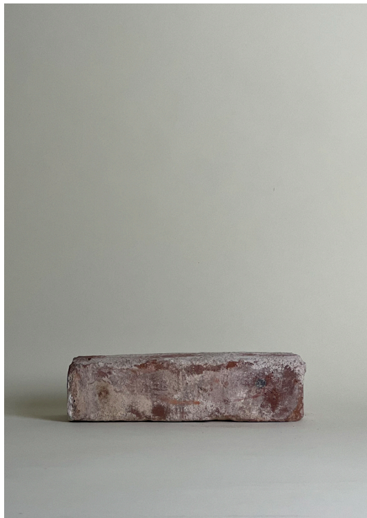
Figure 30, stretchers, height 54 mm x width 228, danish format. From personal collection.
