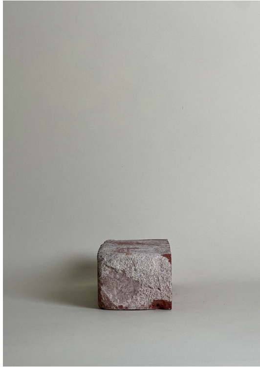
Figure 29, headers, height 54 mm x width 108, danish format. From personal collection.
