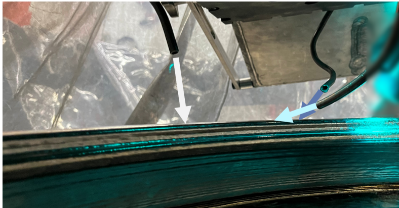
Figure 6.3: Representative illustration of three cooling jets directing cold argon gas onto the newly deposited, hot surface downstream of the laser.
