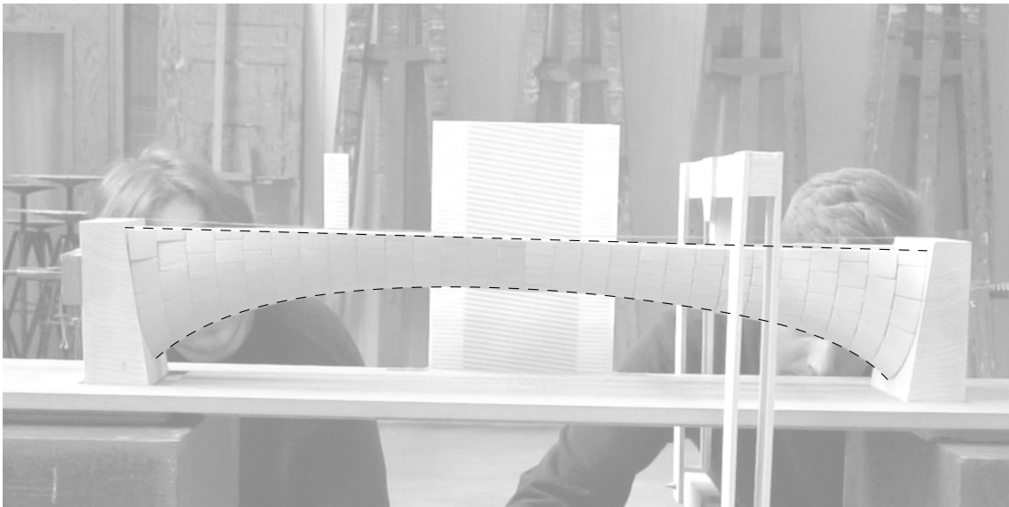
Figure 5.1: Load test of catenary with the load placed at quarter point, loaded with 20 kilograms.
