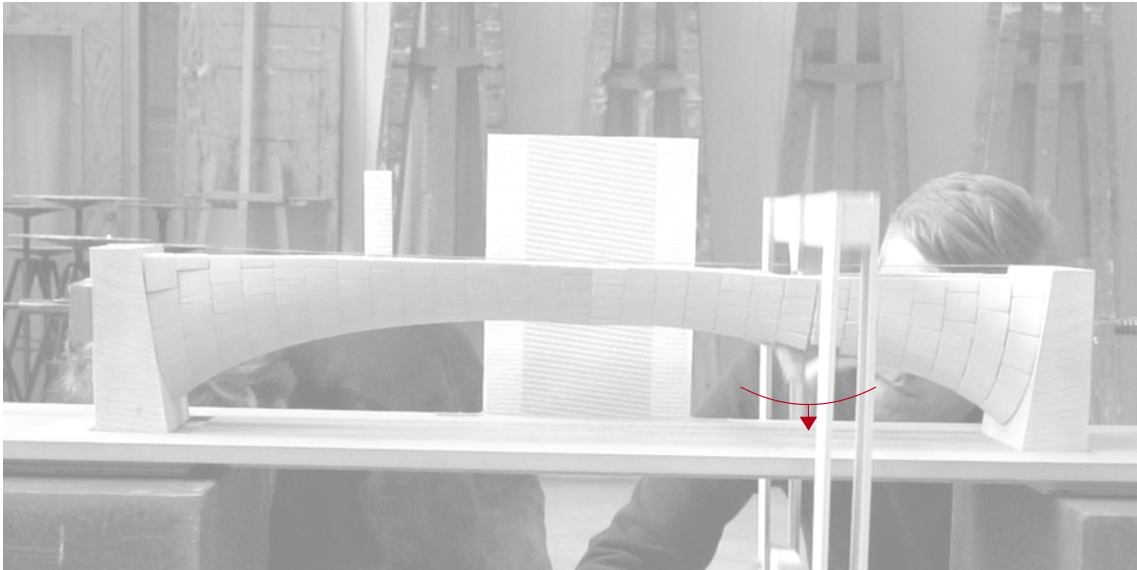
Figure 5.3: Load test of catenary with the load placed at quarter point, collapse at 28.9 kilograms.
