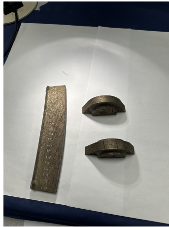
Figure 3.6: Isometric view of mounts and top of part after first cut.
