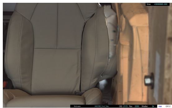
(b) Tear seam beginning to rupture
