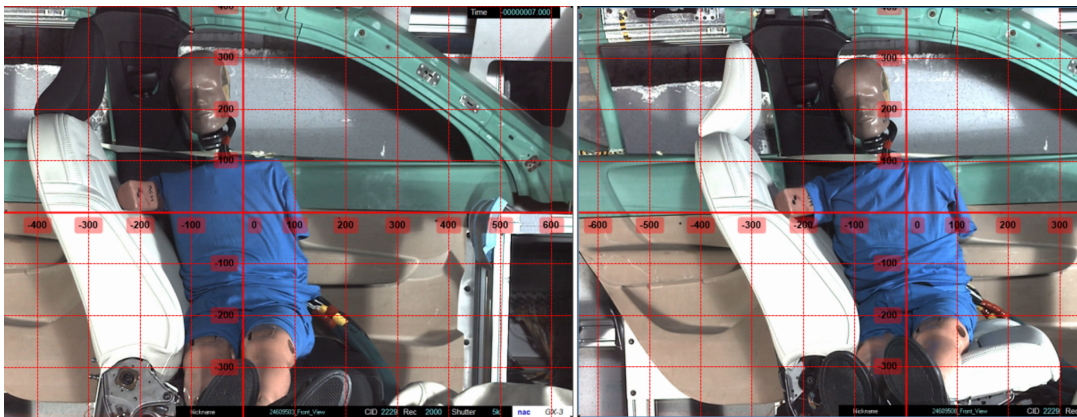
Figure 4.2: Rigid (left) and normal (right) seat structure before signal
