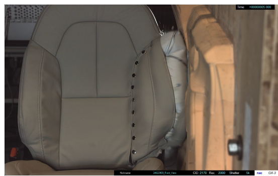
(b) Tear seam beginning to rupture
