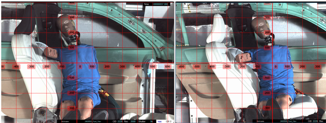
Figure 4.3: Rigid (left) and normal (right) seat structure 37 milliseconds after signal
