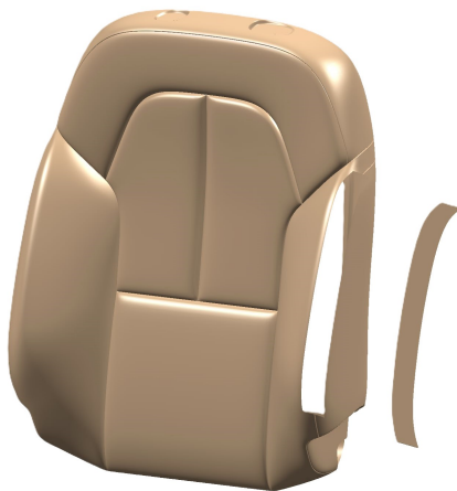
(a) Conceptual model of the replaceable tear seam
