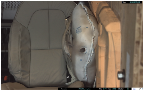
(c) Tear seam completely open
