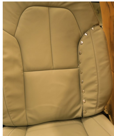
(b) Physical prototype of replaceable tear seam section solution using buttons as connection means
