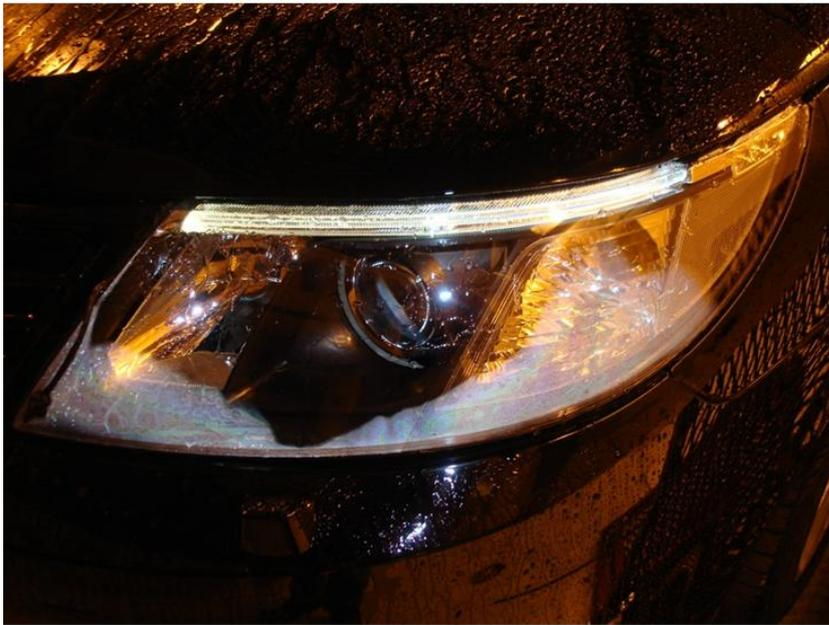
*Figure 1.1 Condensation has taken place on the headlamps outer lens.*
