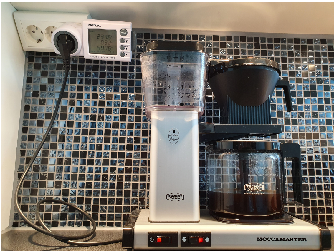
Figure 3.8: Voltcraft logging the energy consumption of a Coffee Maker.
