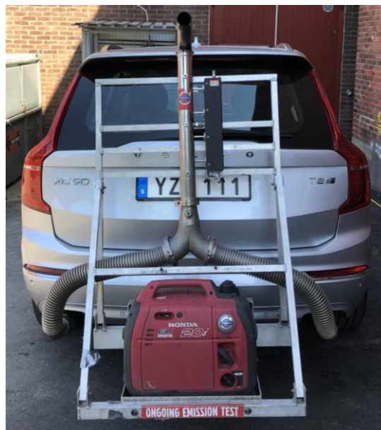
Figure 6. Test Vehicle with Mounting Structure.
