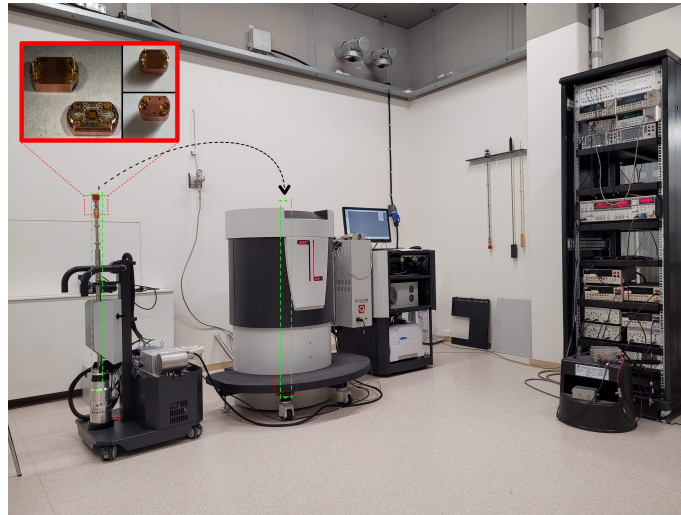
Figure 3.19: A picture of the PPMS setup. The holder is mounted on the RF-stick and inserted vertically into the cylindrical cryogenic chamber.
