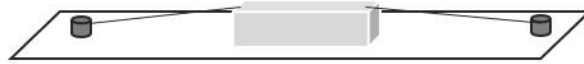
Figure 4.4 Case 1b setup sketch: floating barge in open sea while constrained by two mooring lines.
