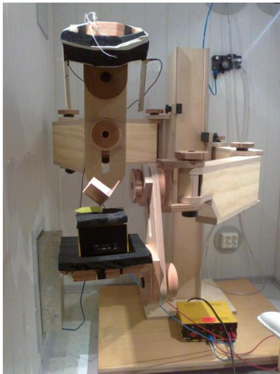
Figure 5-13 Photo of the experimental setup of corner reflector movement detection using the presented UWB radar system.
