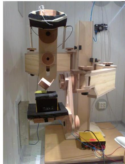
Figure 5. Experimental setup of vibrating corner reflector.
