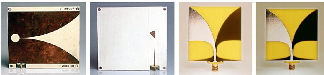
Figure 3-2 Photos of antennas. From left to right: the front side of the Vivaldi 004 antenna; the back side of the Vivaldi 004 antenna; the front side of the Vivaldi 006 antenna; and the back side of the Vivaldi 006 antenna.[11][12]
