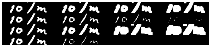
Figure 6: The first two rows show dilation and erosion with a 3 \times 3 kernel and the second two rows show dilation and erosion with a 5 \times 5 kernel.
